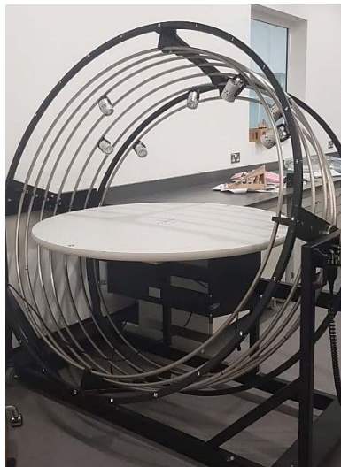
Figure I.2.2.12 One of the equipment (Heliodome) in the Constructional Materials and Building Science Laboratory (B369)
